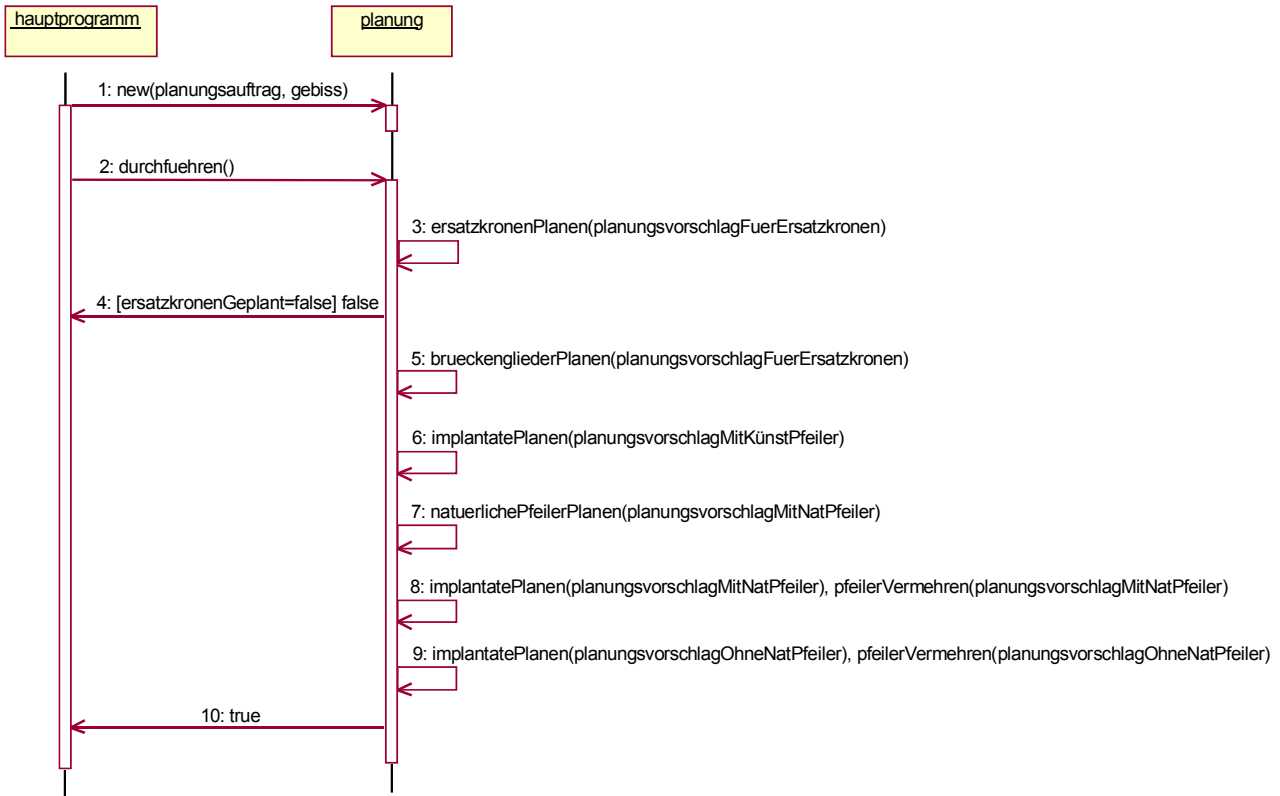
Figure 64: A rough presentation of the sequence diagram for treatment planning. The crown restorations are planned before the necessary abutments, in accordance to the decision model in Chapter 4.
